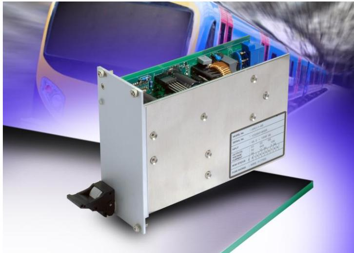
As standard, the triple output CPCIR power supplies operate from 72/110 and 24/36VDC input and provide the following output voltages – 5.1V, 3.3V and 12V. Designed to conform to the standard cPCI profile, these are convection-cooled units that will operate between -40 to +70°C and up to +85 °C for 10 minutes without derating (EN50155 Temperature Class TX).
